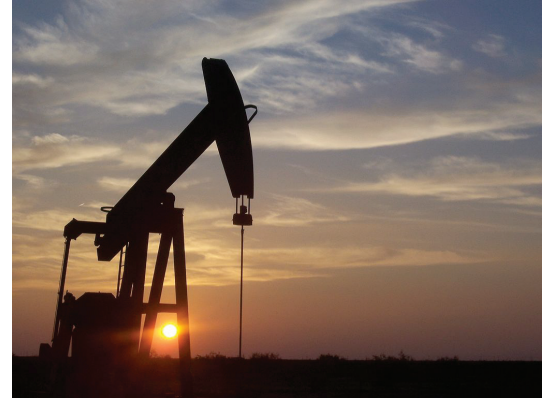
An oil well pump, called a pumpjack, lifts oil from underground to the surface. Oil is a natural resource that is not renewable.
